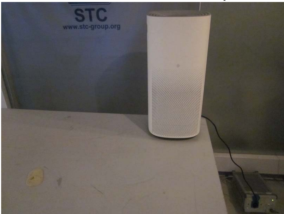
Measurement of Conducted Emission Test Set Up
