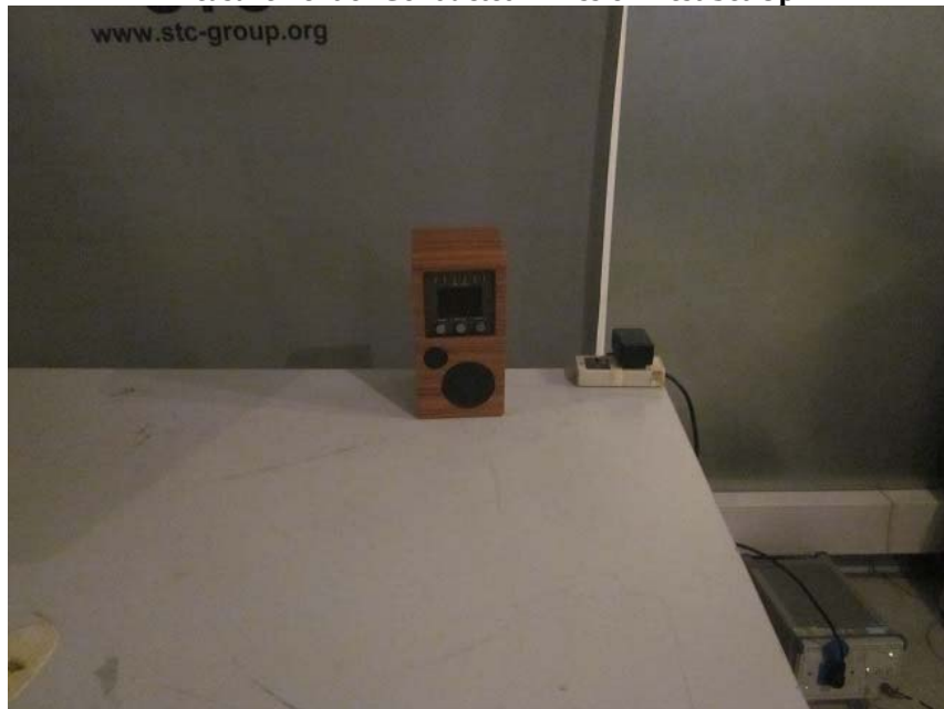
Measurement of Conducted Emission Test Set Up
