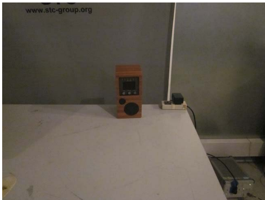
Measurement of Conducted Emission Test Set Up
