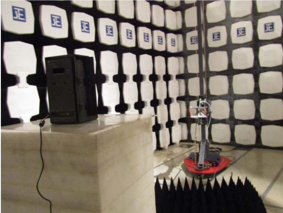
Measurement of Radiated Emission Test Set Up
