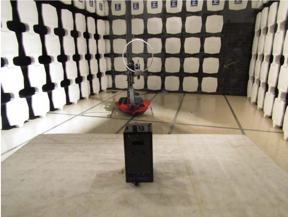
Measurement of Radiated Emission Test Set Up
