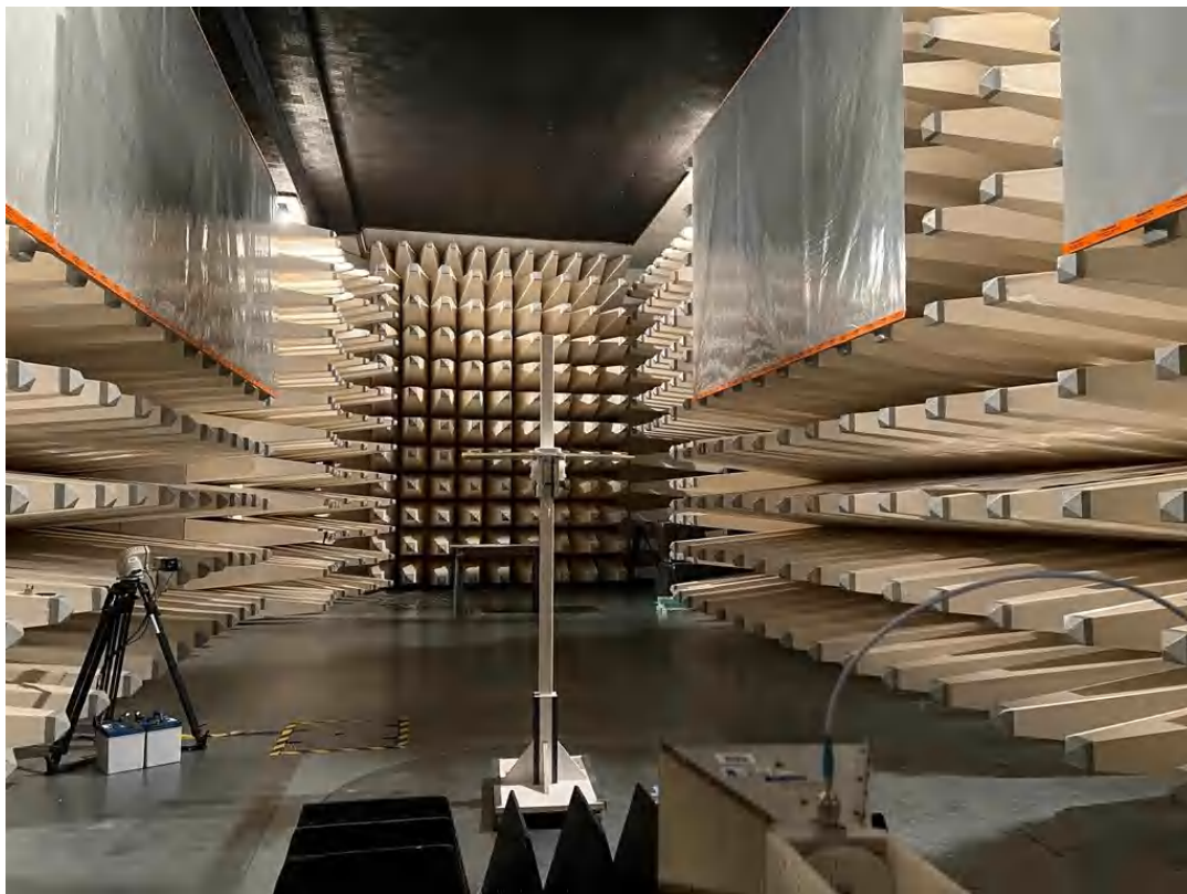
Set up for Radiated Emission Above 1G
