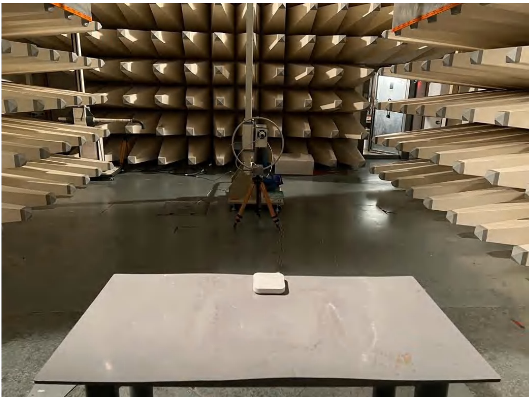
Set up for Radiated Emission Below 30MHz
