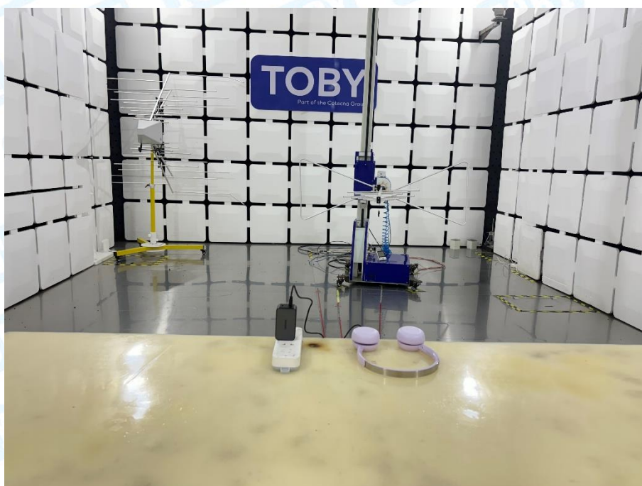
Photo of Setup for Radiated Emission (30MHz~1GHz)
