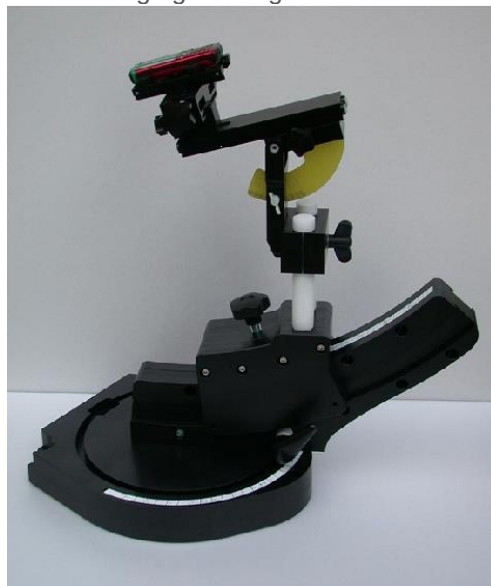
Device holder supplied by SPEAG
