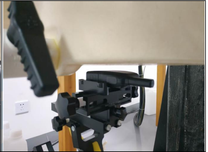
Rear Face of EUT with 1.0 cm Gap
