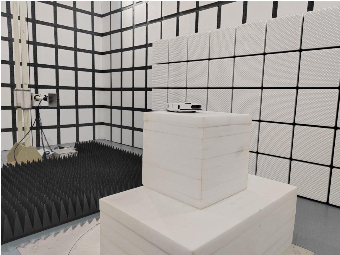
Radiated Spurious Emissions Test Front View (18GHz-25GHz) H1500
