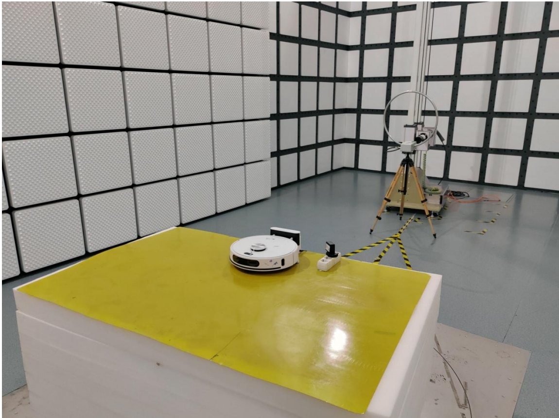
Radiated Spurious Emissions Test View (9kHz-30MHz) H680
