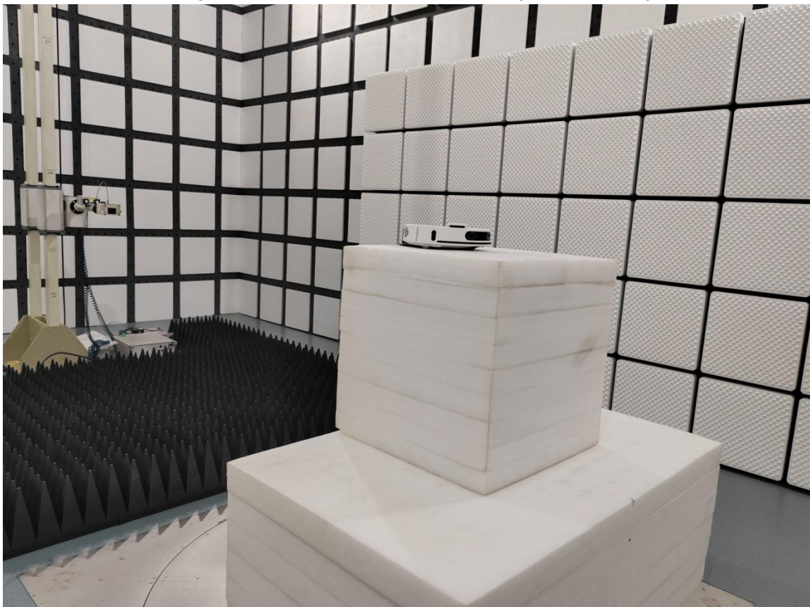
Radiated Spurious Emissions Test Front View (18GHz-25GHz) H1500
