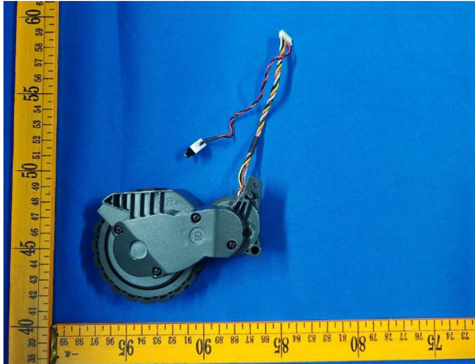
Figure 15. Alternative Wheel motor: RS520-15420 of Robotic Vacuum Cleaner
