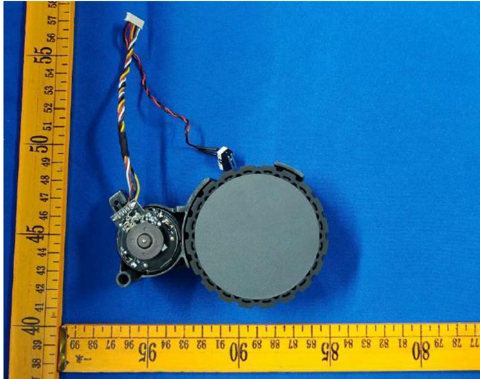
Figure 14. Alternative Wheel motor: RS520-15420 of Robotic Vacuum Cleaner
