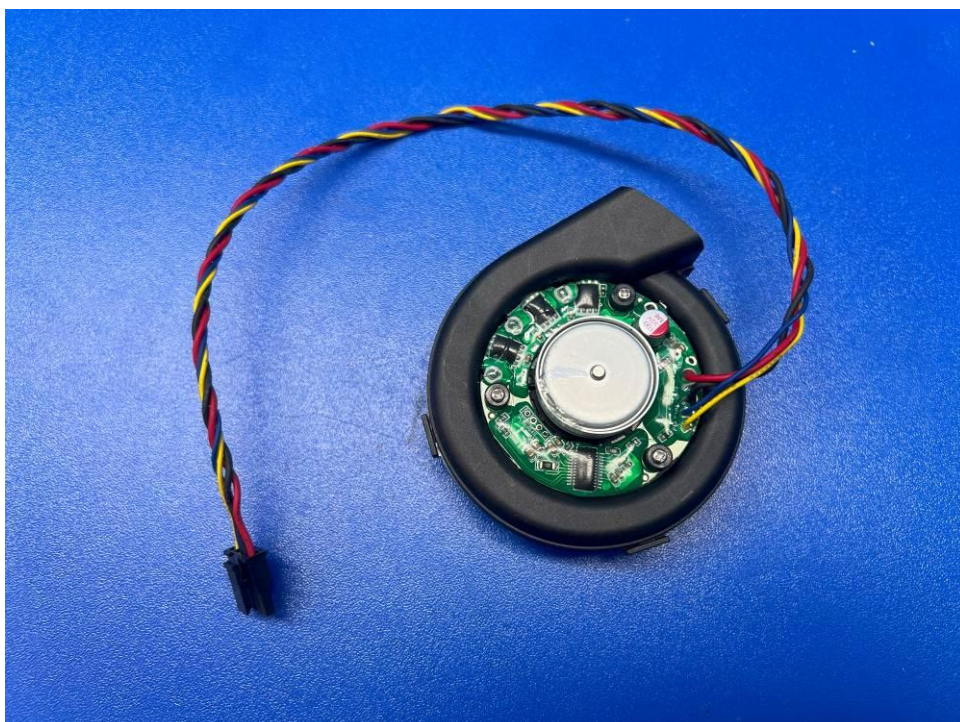
Figure 13. Alternative Suction motor: QYC20A16F-68 of Robotic Vacuum Cleaner
