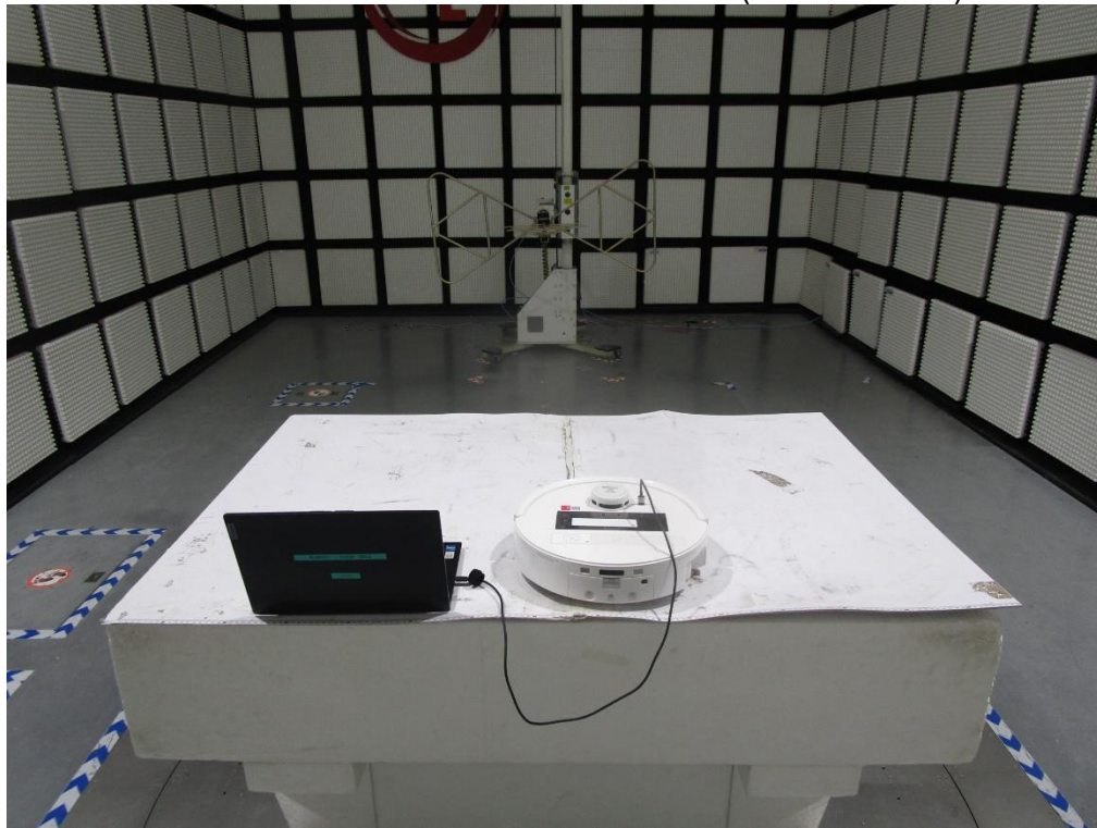
RADIATED RF MEASUREMENT SETUP (Below 30MHz)
