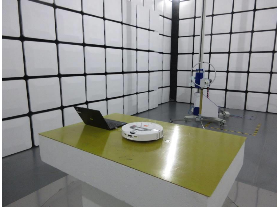
RADIATED RF MEASUREMENT SETUP (9kHz ~ 30 MHz)
