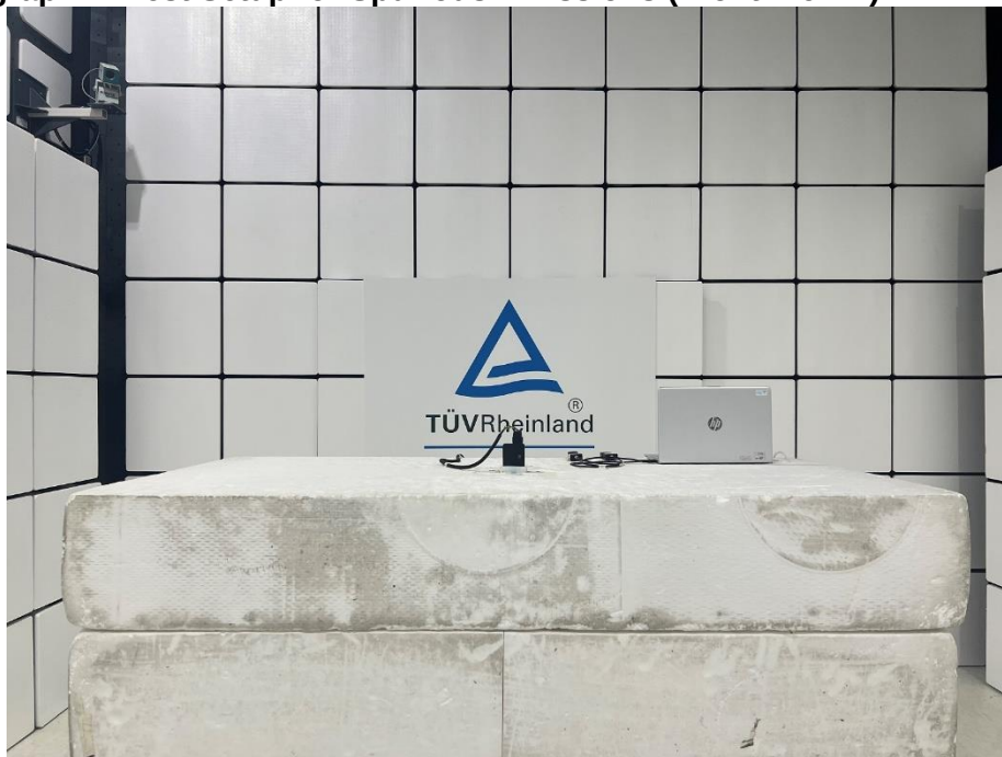
Photograph 2: Test Setup for Spurious Emissions (Front View 2)
