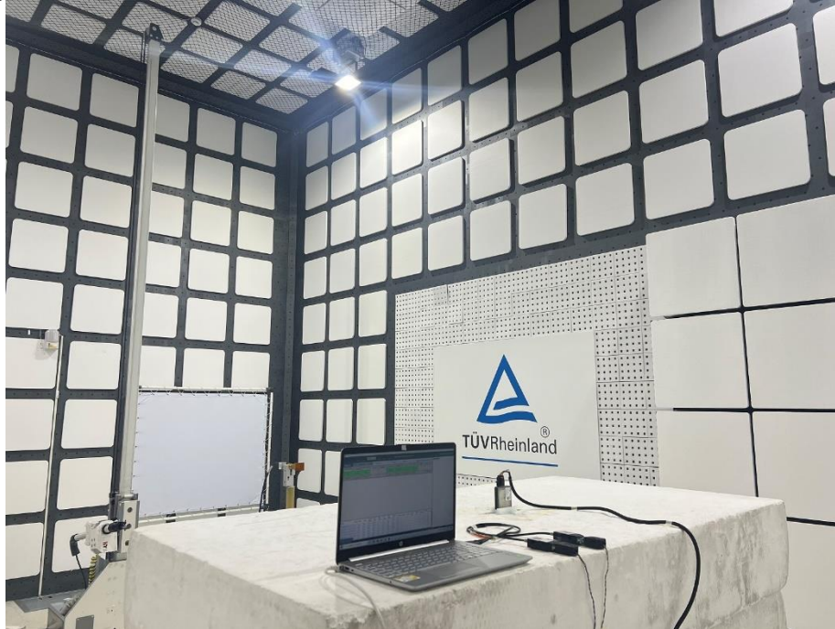
Photograph 8: Test Setup for Spurious Emissions (Back View 6)
