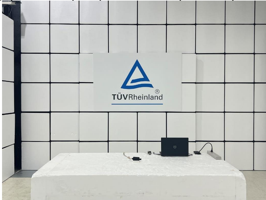
Photograph 2: Test Setup for Spurious Emissions (Front View 2)
