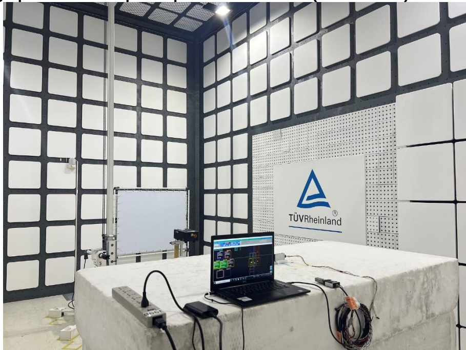
Photograph 8: Test Setup for Spurious Emissions (Back View 6)
