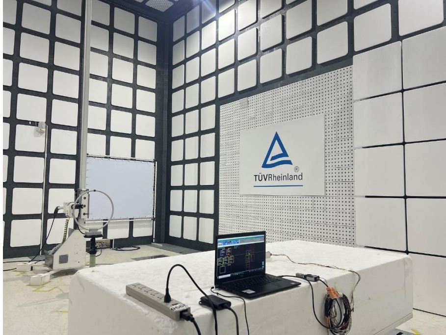
Photograph 3: Test Setup for Spurious Emissions (Back View 1)
