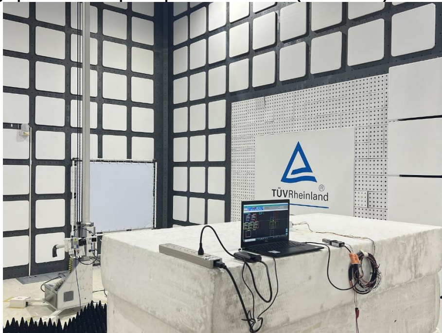
Photograph 6: Test Setup for Spurious Emissions (Back View 4)
