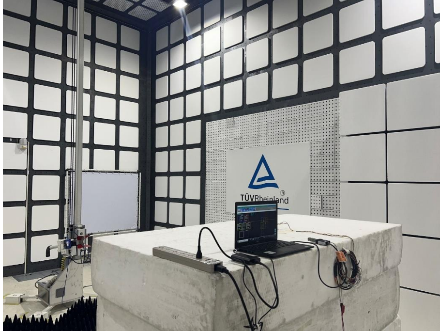
Photograph 5: Test Setup for Spurious Emissions (Back View 3)
