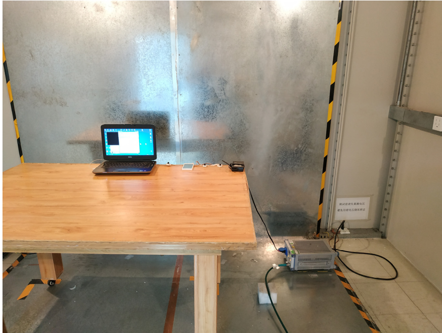
Conducted Emissions (Side View)
