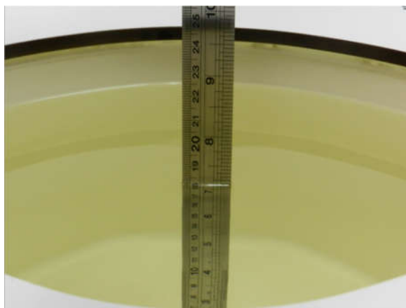
Fig 10.2 Photo of Liquid Height for Body SAR
