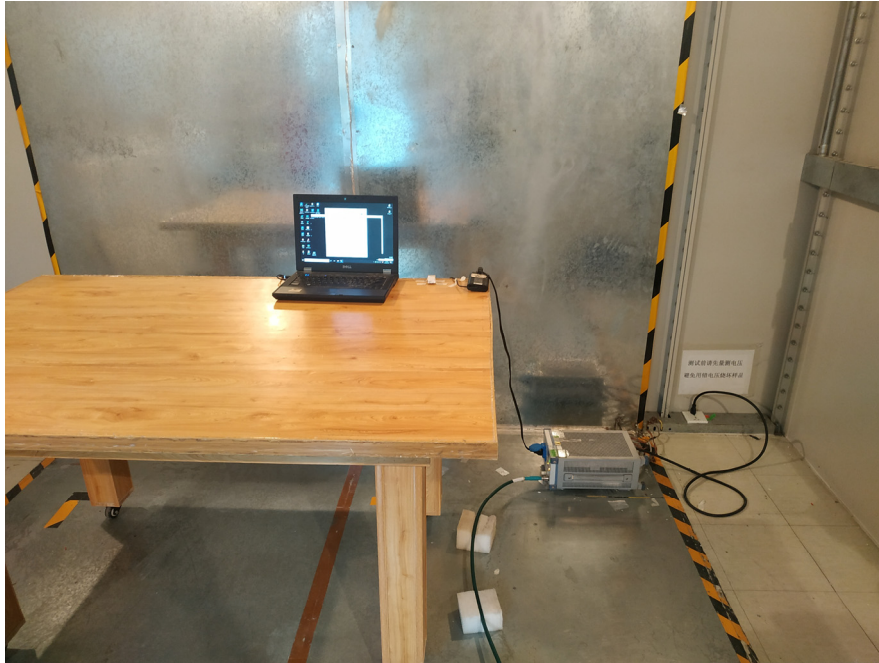
Conducted Emissions (Side View)
