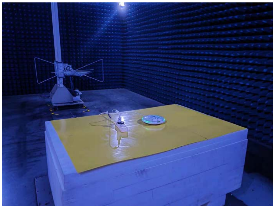
Photo of Radiated Emission Measurement Below 1GHz
