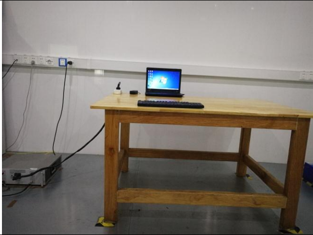
Conducted Emissions Test Setup Front View
