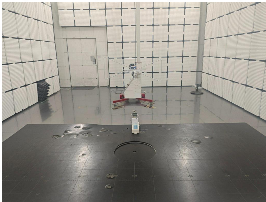
Radiated emissions (30MHz-1GHz)
