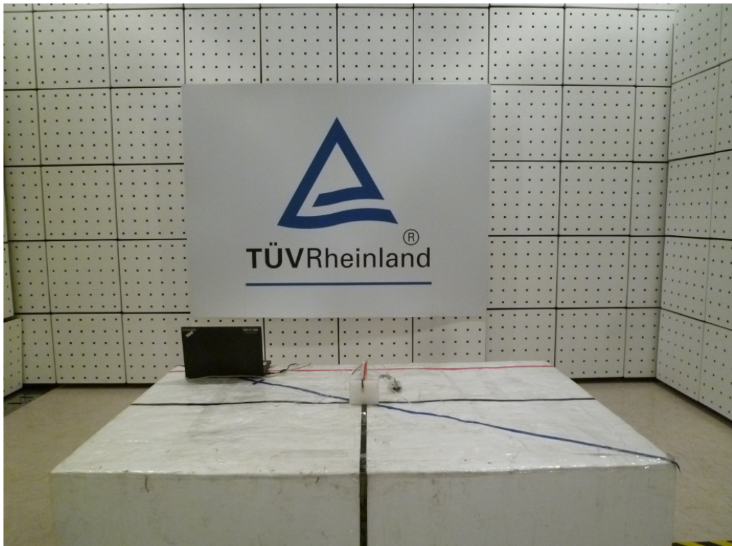
Photograph 1: Set-up for Spurious Emissions (Front View)
