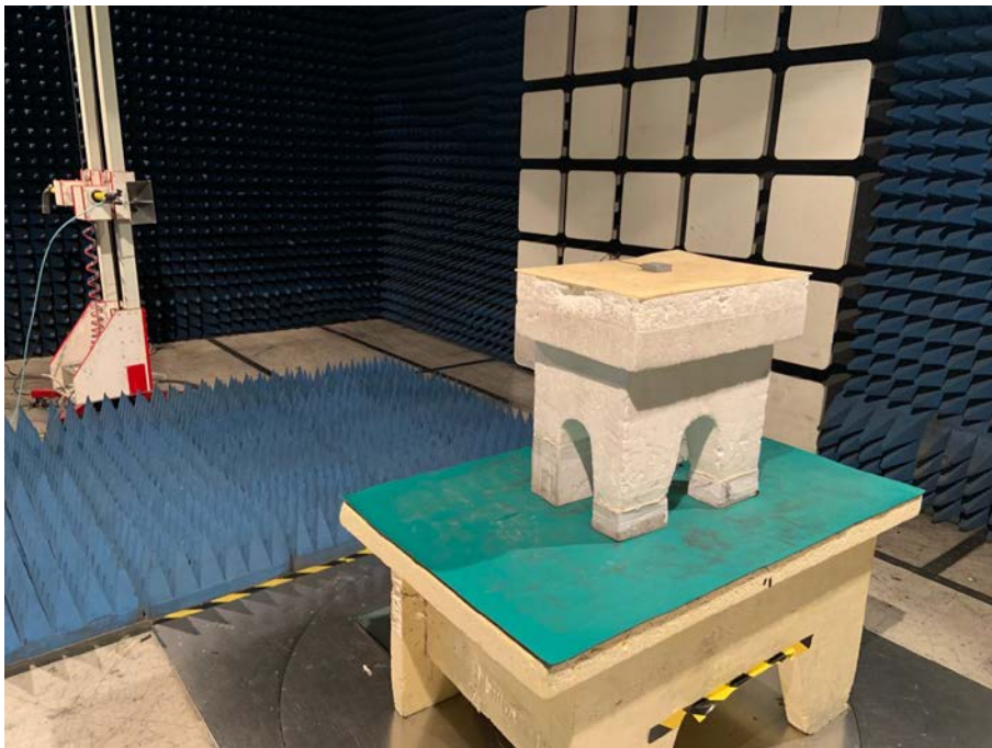
Spurious Emission Test Setup (Above 1GHz)
