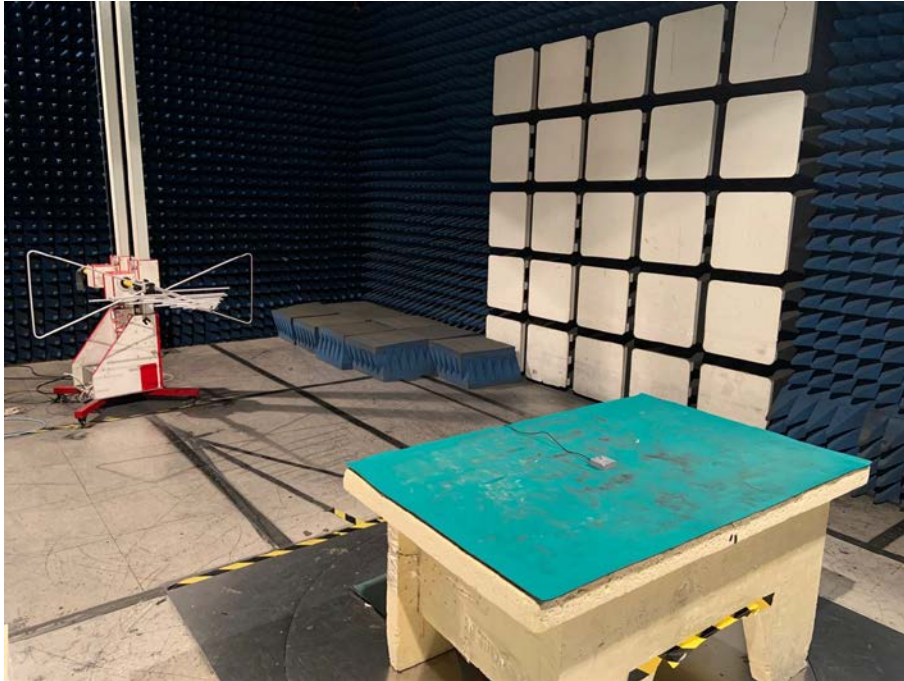
Spurious Emission Test Setup (Below 1GHz)
