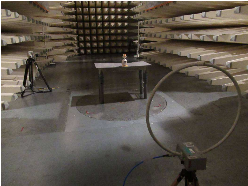
Setup for Radiated Emission (Bluetooth Low Energy)
