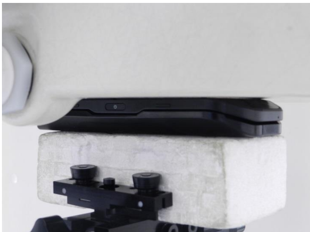
Front with Battery Pack, Test Separation 0 mm
