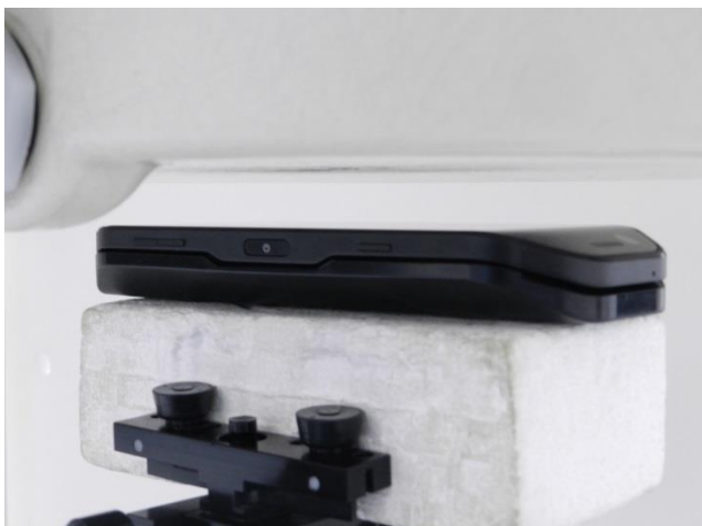
Front with Battery Pack, Test Separation 15 mm
