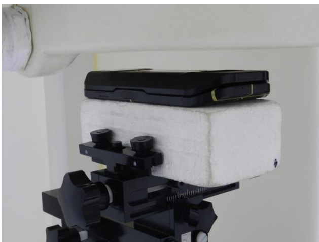
Back with Battery Pack, Test Separation 15 mm
