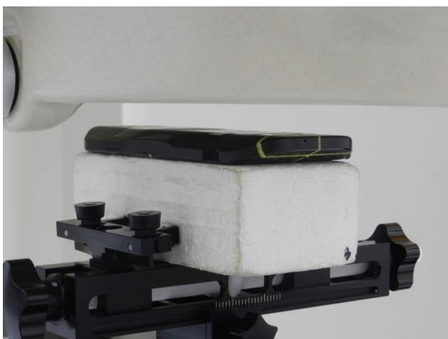
Back, Test Separation 15 mm
