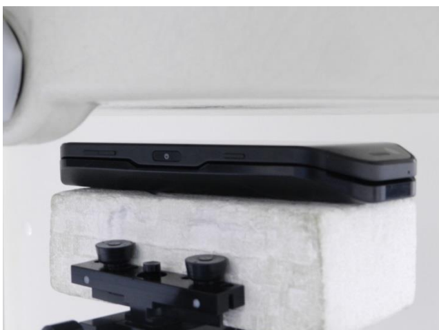
Front with Battery Pack, Test Separation 15 mm
