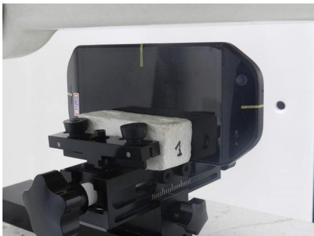
Left Side, Test Separation 10 mm
