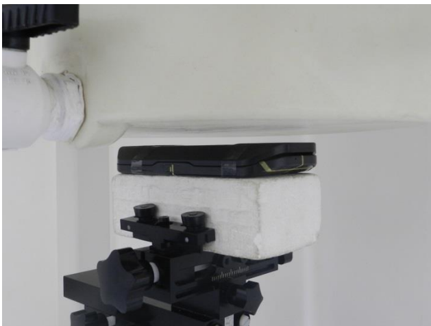
Back with Battery Pack, Test Separation 10 mm
