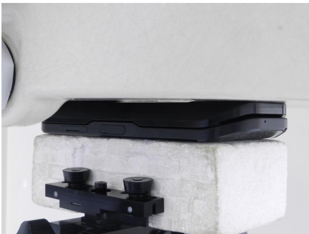
Back with Battery Pack, Test Separation 0 mm
