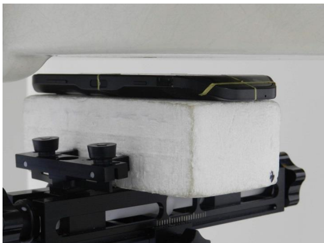
Front, Test Separation 10 mm
