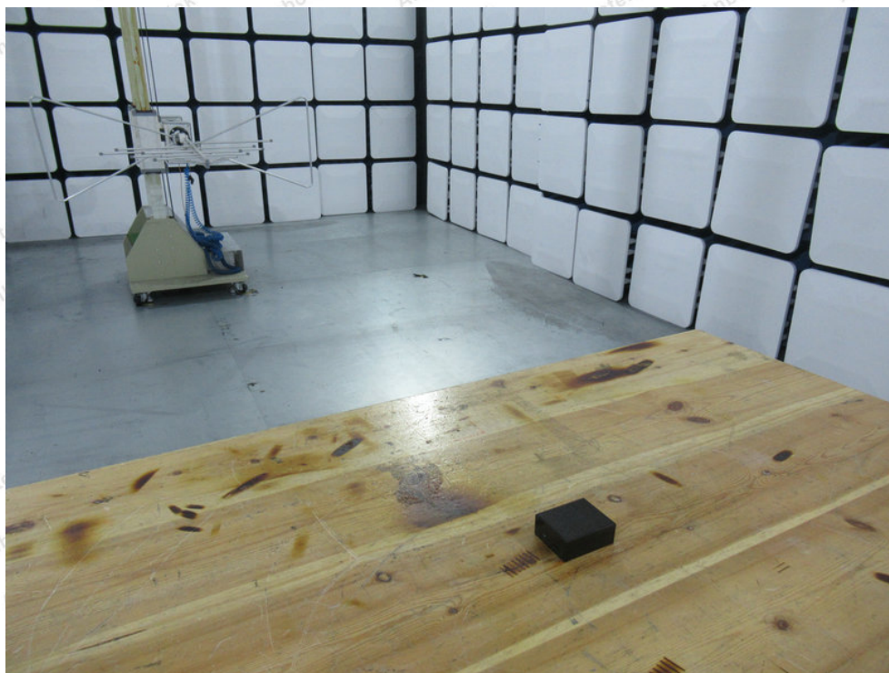
Photo of Radiation Emission Test
