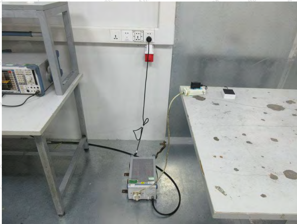
Photo of Conducted Emission Measurement
