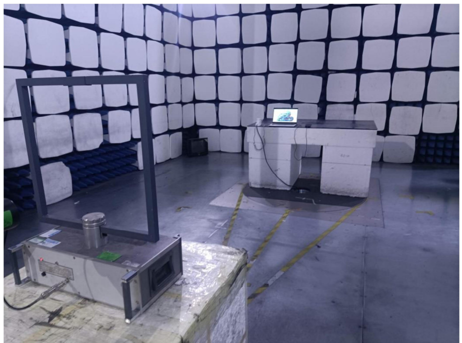
Radiation Emission Test Setup (Below 30MHz)
