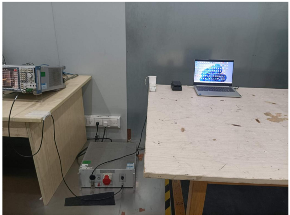
Conducted Emission Test Setup
