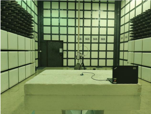
WLAN 5G Radiated Setup Change Antenna Layout
