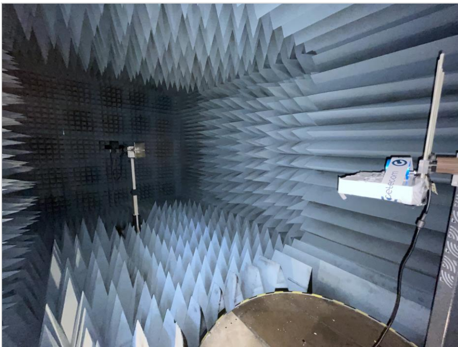
Photograph 6: EUT test setup in the fully anechoic chamber. Tested frequency 1-17 GHz
