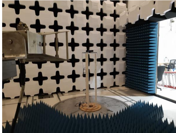
Figure 42: REE Test Setup - 1-18 GHz
