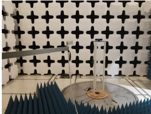
Figure 43: REE Test Setup - 18-25 GHz
