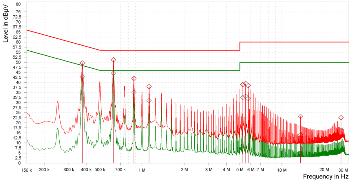
Plot No. 6: Conducted emissions, set-up 2, Op. 1, N
