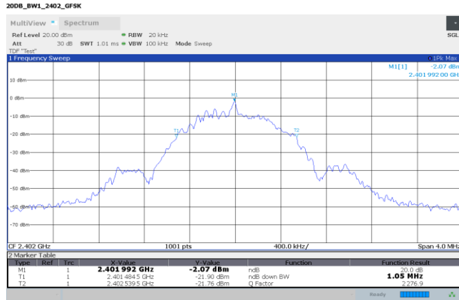
Figure 8.2-1: 20 dB occupied bandwidth, 2402 MHz
