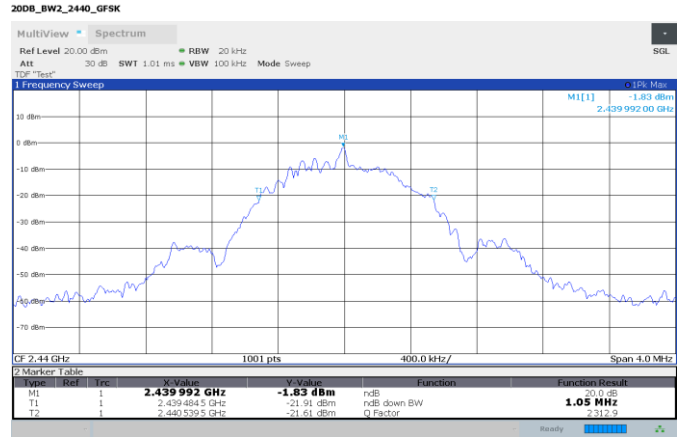
Figure 8.2-2: 20 dB occupied bandwidth, 2440 MHz
