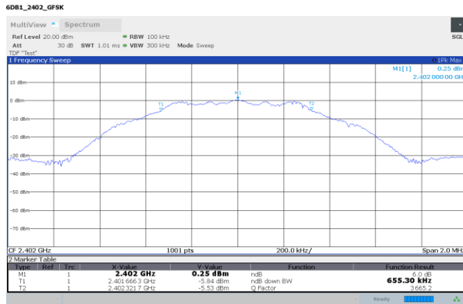
Figure 8.3-1: 6 dB DTS bandwidth, 2402 MHz
