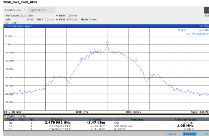
Figure 8.2-3: 20 dB occupied bandwidth, 2480 MHz
