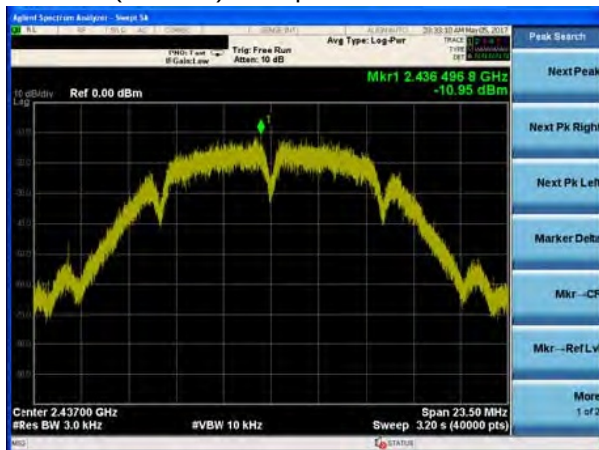
(802.11b) PSD plot on channel 6
