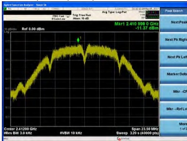
(802.11b) PSD plot on channel 1
