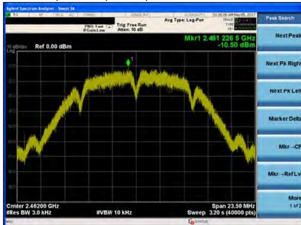
(802.11b) PSD plot on channel 11
