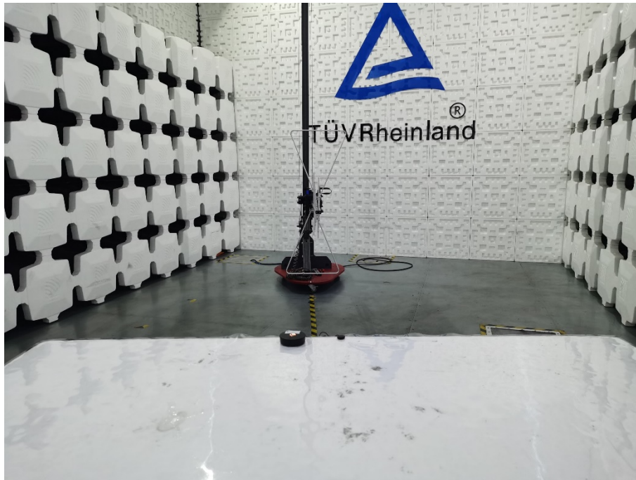
Photograph 4: Set-up for Radiated Emission, Above 1GHz
