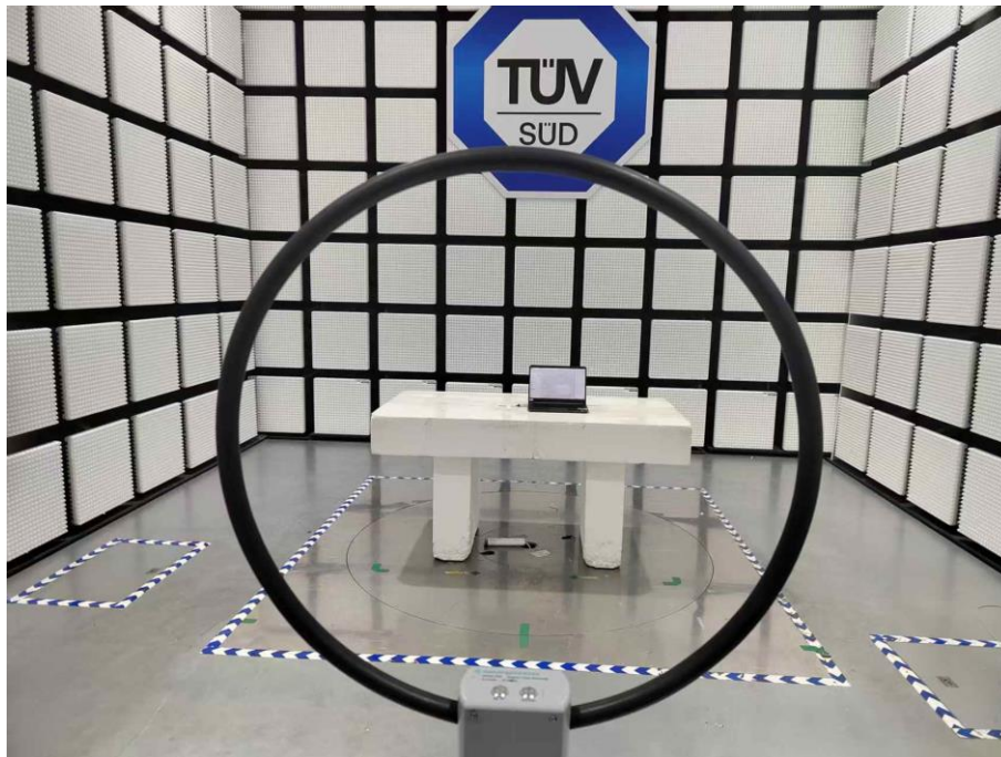
Radiated Emission Setup 9kHz ~ 30MHz
