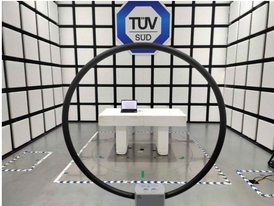
Radiated Emission Setup 9kHz ~ 30MHz
