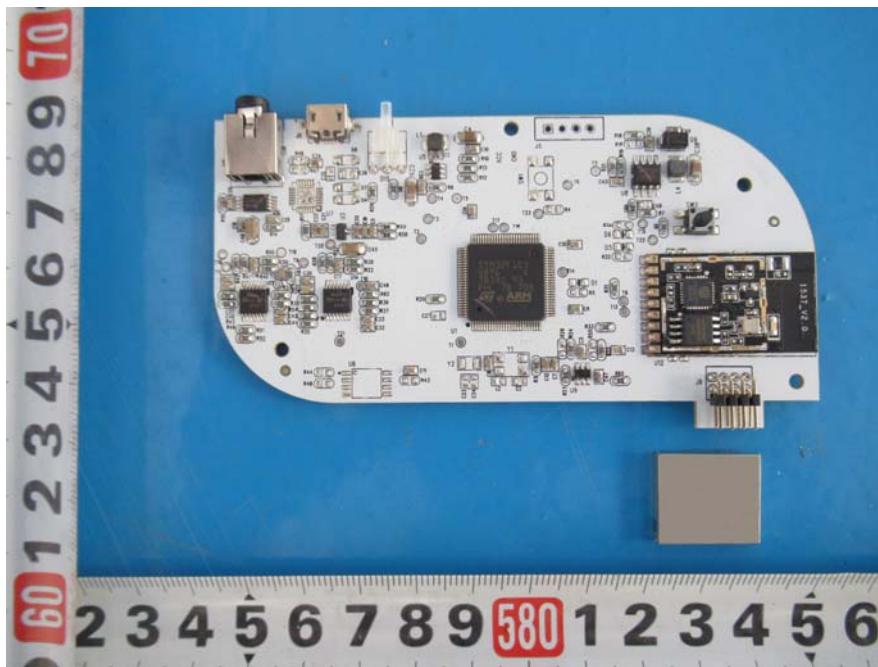
EUT – PCB-1 Bottom View
