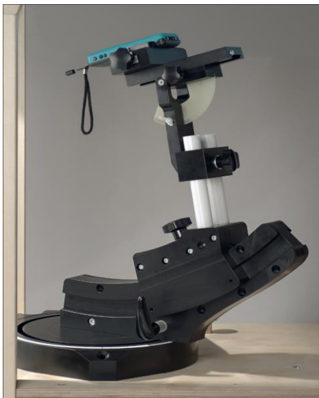
F-2. Device Holder for Transmitters
