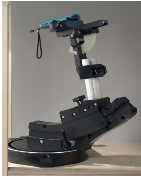
F-2. Device Holder for Transmitters
