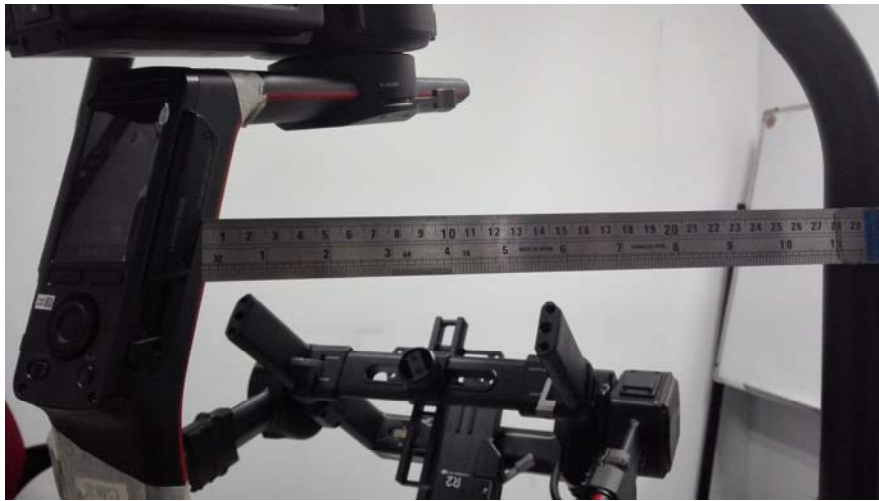
EUT – Handle to Antenna distance View (27.5 cm)
