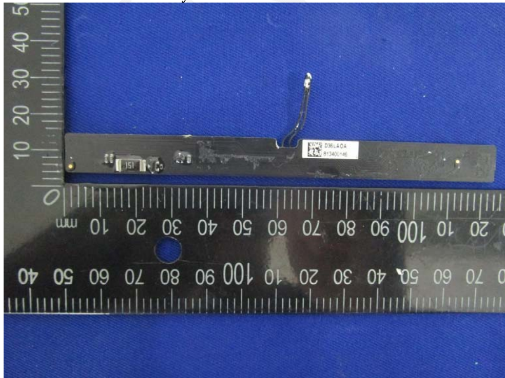
EUT – Battery Power Control Board Bottom View
