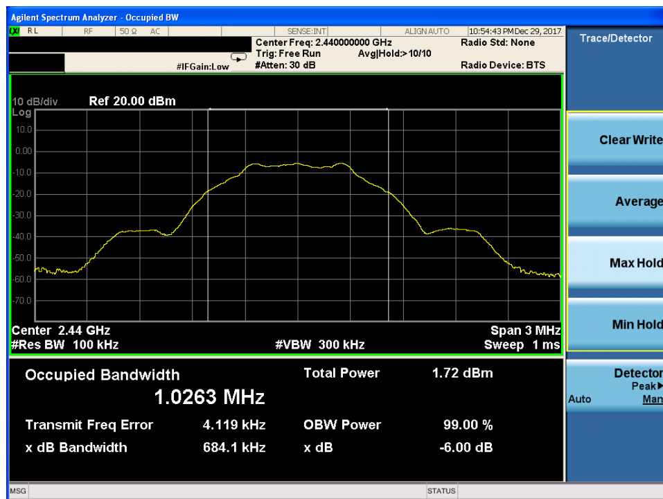
6dB Bandwidth plot on channel 19
