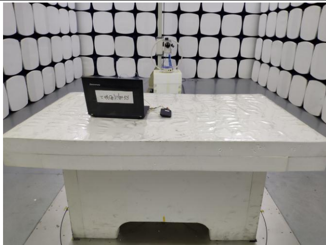
Radiated Emissions Test Setup Below 30MHz
