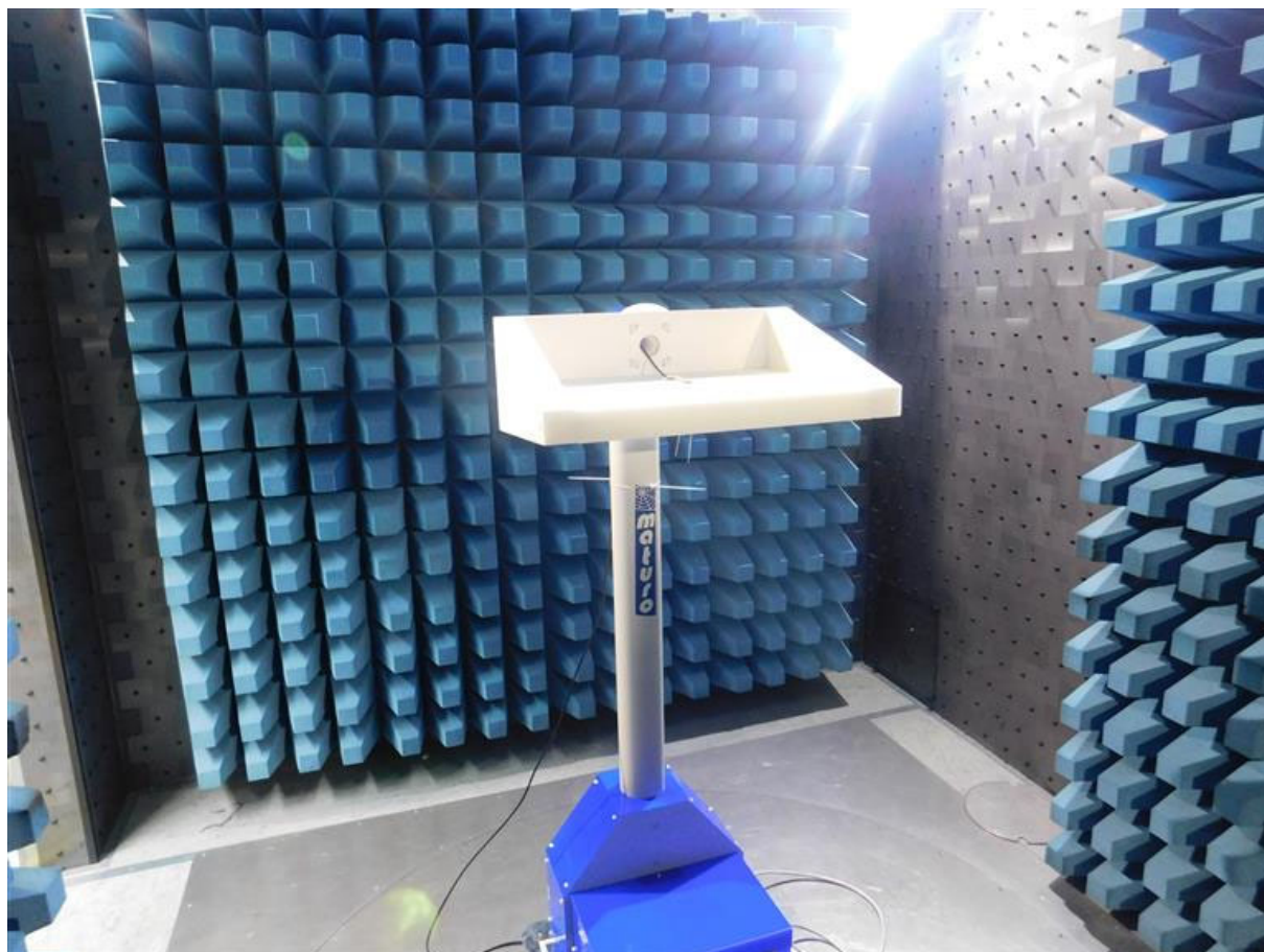
Figure 2 : Test set up Antenna Measurement
