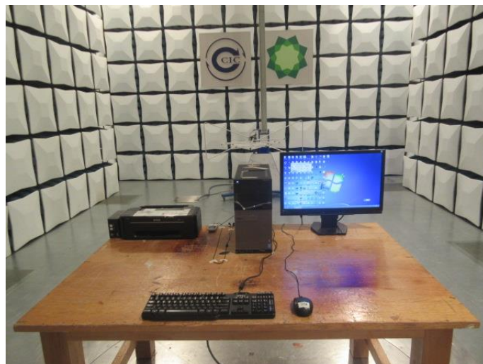
Radiated Emission (above 1GHz) Connect to PC
