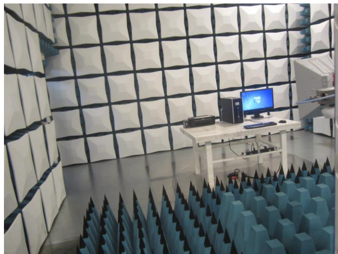
Radiated Emission (above 1GHz) Connect to PC
