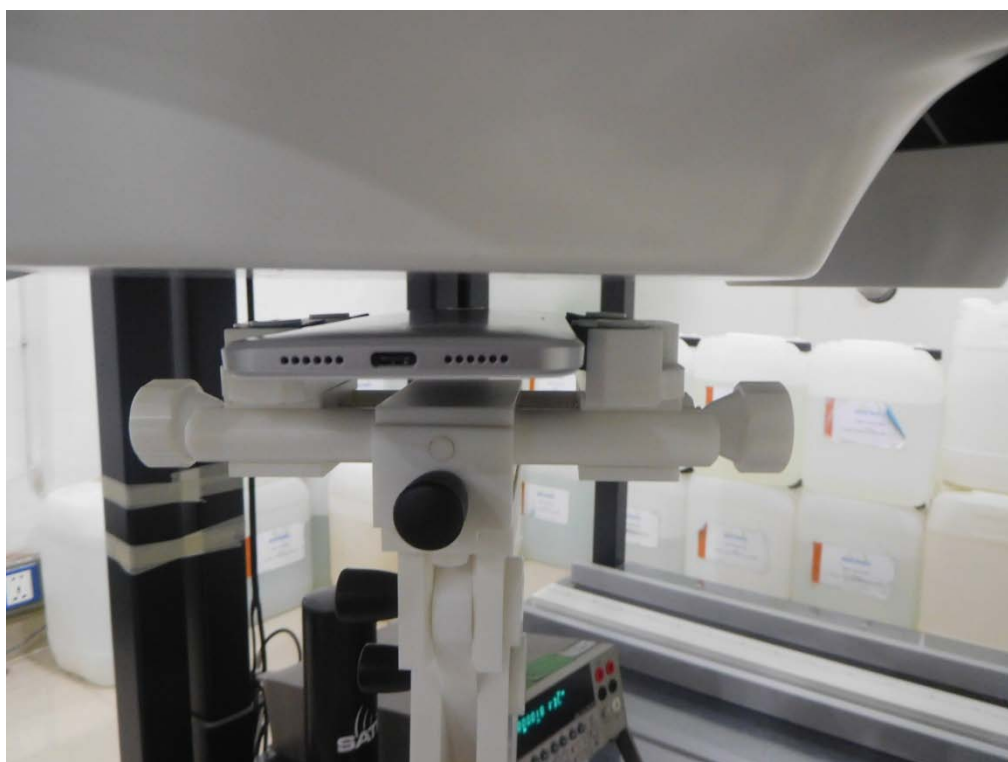
Body Back side(separation distance is 10mm)
