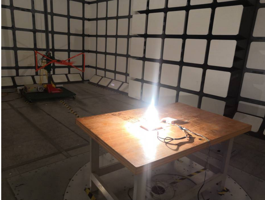
Radiated Emissions View (Below 1 GHz)
