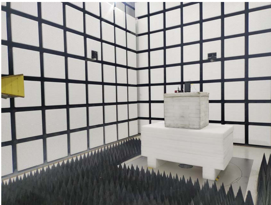
Radiated Emission Above 1GHz View
