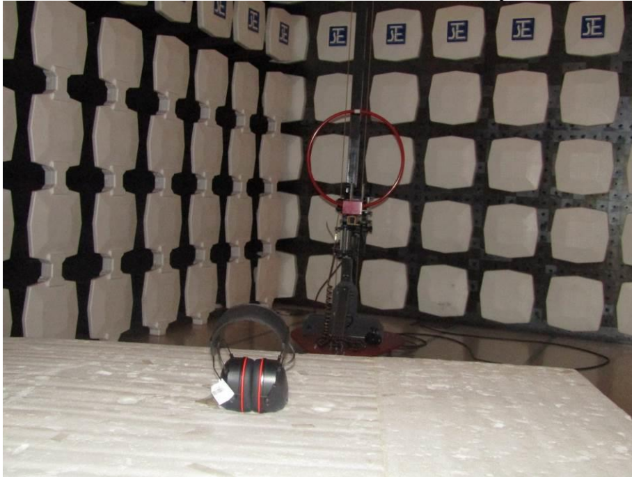
Measurement of Radiated Emission Test Set Up
